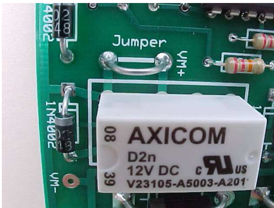
Figure 9. Install the jumper on the board if you are using a 12 VDC motor.
