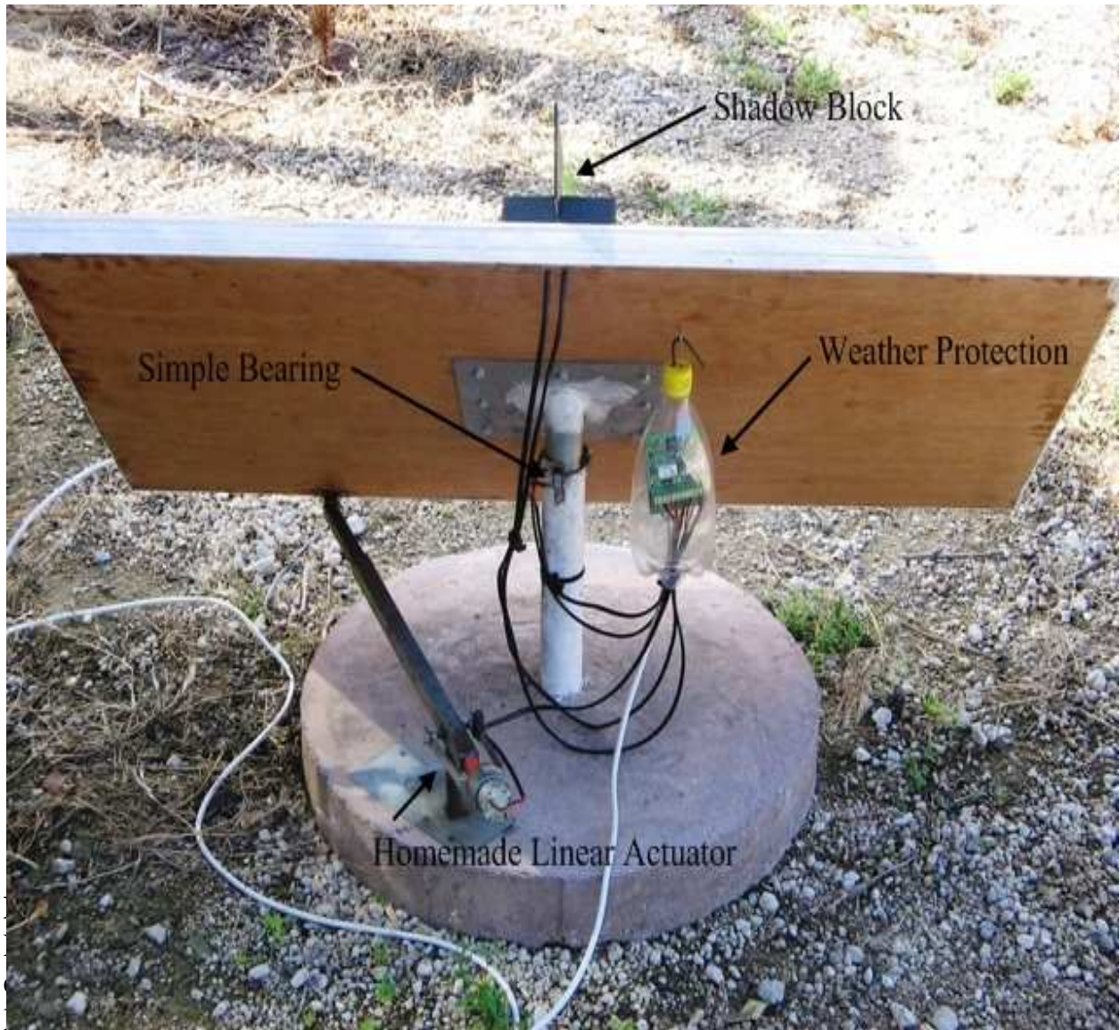
Figure 35. This Solar Tracker Project uses a DC linear actuator to move the panels. The controller is mounted inside a weatherproof electrical enclosure. The photos are courtesy of Bill F.
