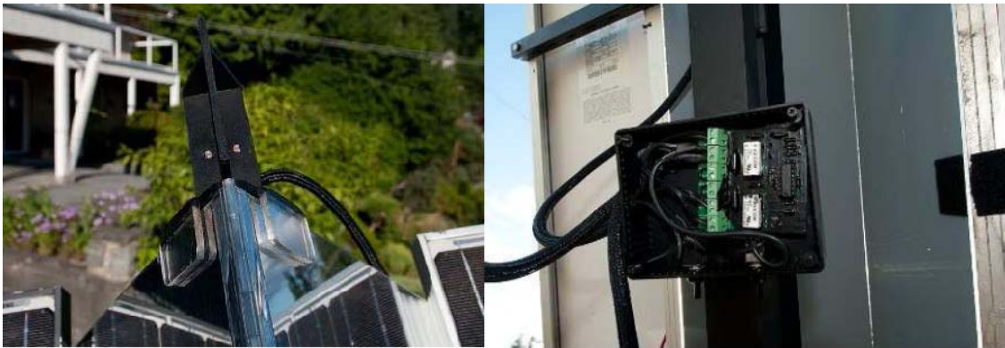
Figure 38. Here is a view of the same tracker from Figure 33. Note the the shadow block assembly. Also, note how the circuit board was ruggedized with a conformal coating and is mounted in a weather tight enclosure.
