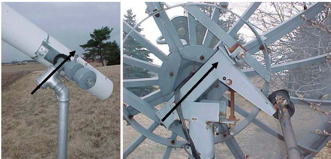
Figure 3. Examples of mechanical mounts aligned to the polar axis.
