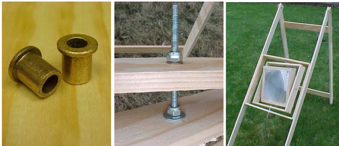
Figure 23. Flanged sleeve bearings used with a simple Fresnel Lens tracker.
