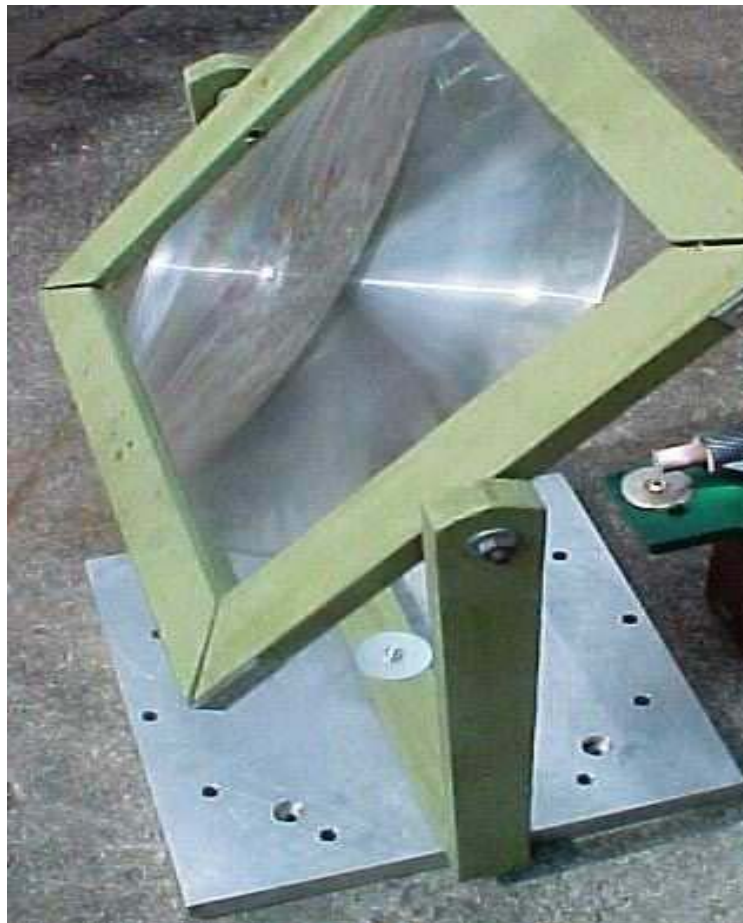
Figure 33. Fresnel lens powering a small air cycle stirling engine.
