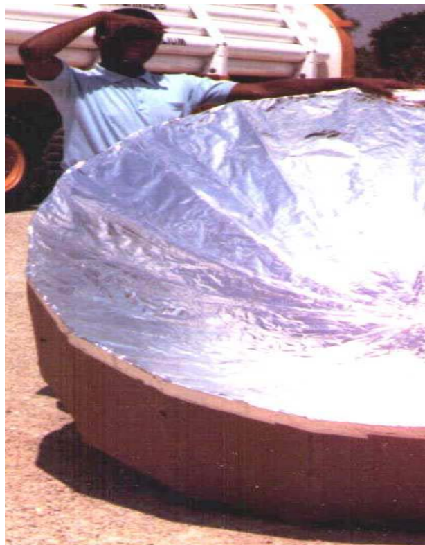
Figure 32. Example of a spherical reflective collector built using cardboard and aluminum foil. A typical example of a transmissive type solar concentrator is a glass lens. The lens focuses the light to a single spot, also called the focal point. Glass lenses tend
