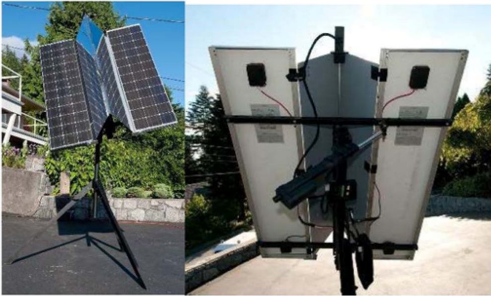
Figure 37. This awesome Solar Tracker project is the work of David. Note the use of a central mirror reflector to increase sunlight on the panels. These panels are moved with a heavy duty linear actuator.
