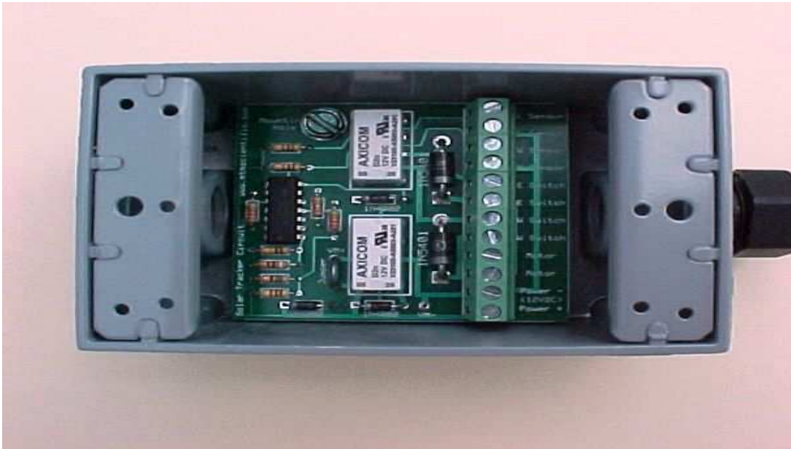
Figure 12. The Solar Tracker circuit board fits inside a standard outdoor box. Be sure to insulate the bottom of the board from making metallic contact.
