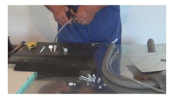
I put a piece of hose on the steel sheet, I will get the wires through that and I don't want the sharp edge to cut through the wire.
