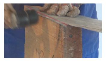
To obtain a nice and rounded shape, I will use a steel pipe and the hammer to model the cone.
