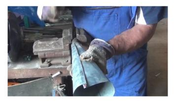
I cut the excess material from both sides using the angle grinder.
