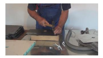
From a rubber hose, I cut some pieces to insulate the screws from the steel wool.
