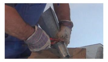
To shape the cone even further, I will secure the steel pipe in the vise and round the straight edges that have formed when bending the material.
