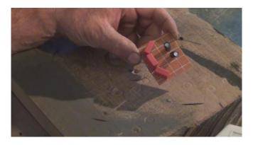
2 diodes and 2 x 50 V polarized capacitors connected in series.
