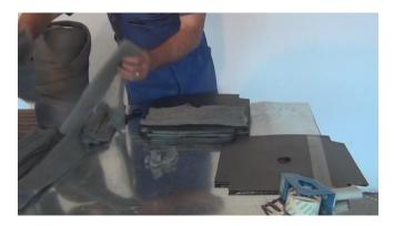
I create a template for the holes on one of the bitumen protection layers so I can insert screws for securing the layers to the lid.
