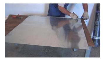
After doing that, I cut the excess from each corner and obtain the unwrapped 5 sides of the cube.
